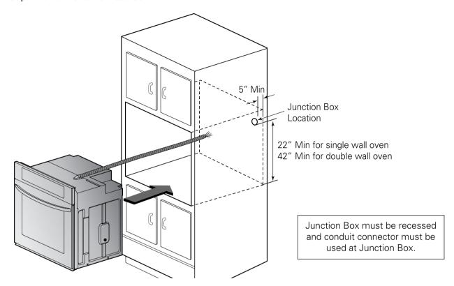
3. If local codes permit connection of the frame grounding conductor to the neutral(white) wire, follow the instruction of 3-wire circuit connection on page 10.
